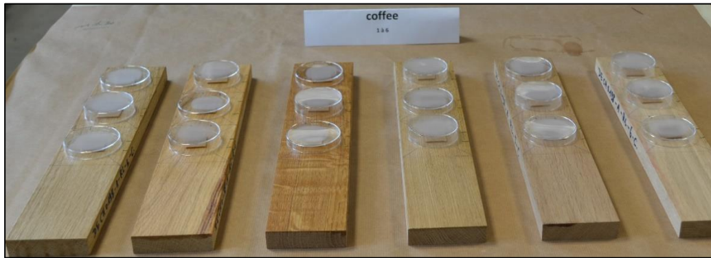
Photo 1: the six types of wood paint with the coffee stain agent under a petri dish
