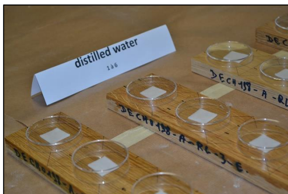
Photo 2: detail of the water stain agent applied on the test surfaces
