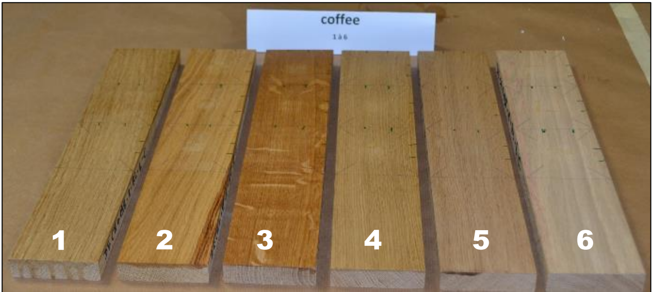
Photo 5: results of the staining test with coffee on DE-CH-0198-A-1 (1), DE-CH-0198-A-2 (2 DE-CH-0198-A-3 (3), DE-CH-0198-A-4 (4), DE-CH-0198-A-5 (5) & DE-CH-0198-A-6 (6).
