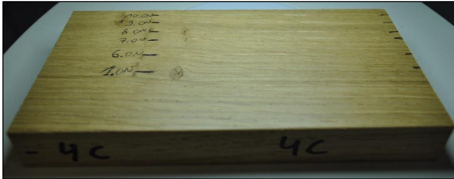
Photo 7: test piece DE-CH-0198-RS-4-C - result of the scratch test
