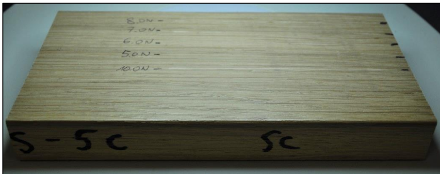
Photo 8: test piece DE-CH-0198-RS-5-C - result of the scratch test
